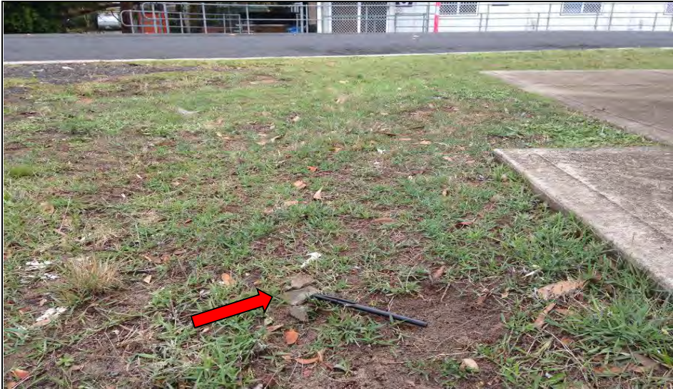
Photo 2: Suspected asbestos containing fibre cement fragment near gas storage facility in Norville Depot.
